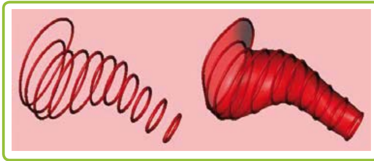
Figure 7: Section curves and loft surfaces.
