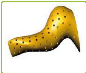
Figure 11: Shell CAD model of an innovative solution for venting paths
