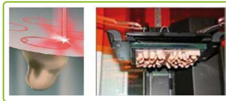
Figure 5 The shell is produced by a Direct Digital Manufacturing System in a bio-compatible material..
