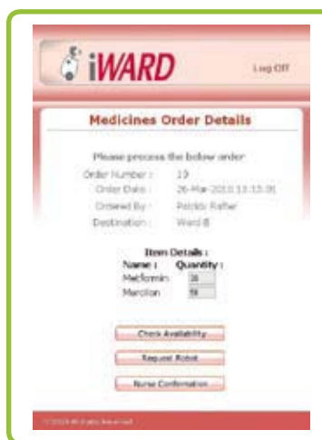
Figure 8: GUI/TUI for action selection: user can choose to check the availability, accept or modify the order before proceeding, i.e. ordering the delivery robot.
